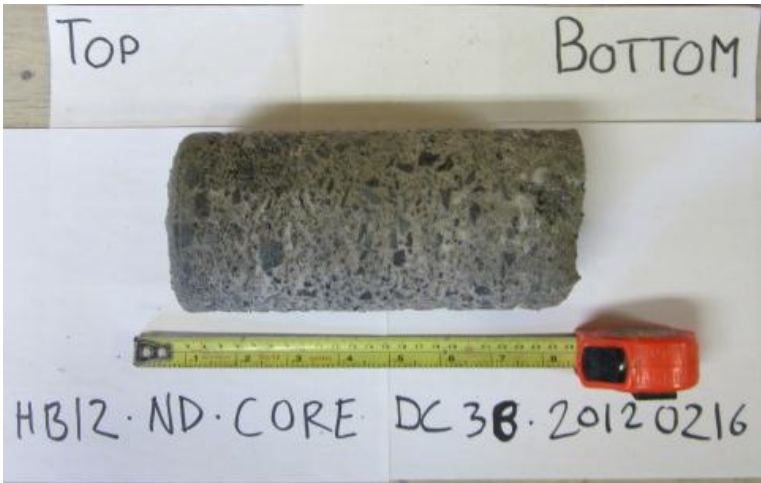
Photo 5: Drill core quality has improved since new core barrels have arrived on site.
