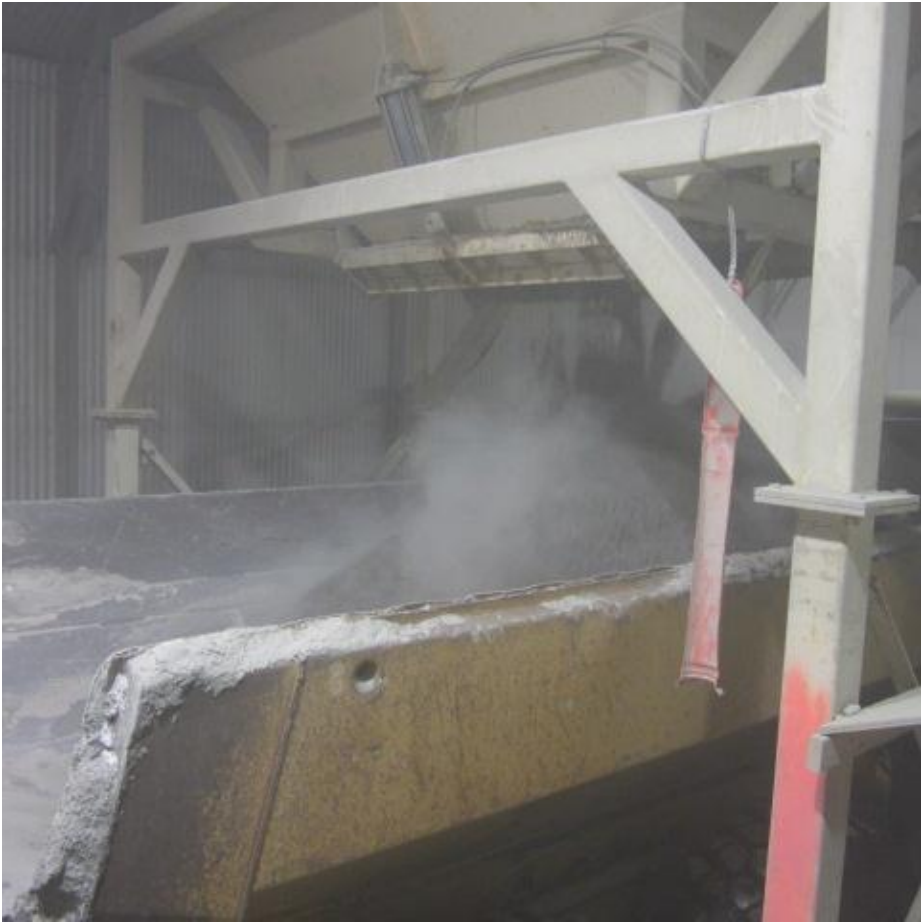
Photo 3: Photo of a haul truck being loaded under the surge bin. The new material requires more moisture to achieve saturation. The angle of repose is flatter than previous 20mm FCM.
